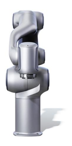
Diana 7 is an industrial lightweight seven-axis robot. With a payload capacity of seven kilograms and a functional reach of 923 mm it is particularly suitable for complex and highly sensitive assembly processes, as a torque sensor is installed in each joint.
