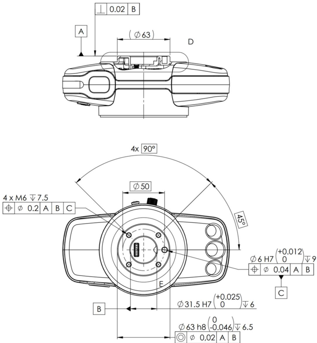
Fig. 10 Dimensions of mechanical interface on the media flange, view 1 (dimensions in mm)
