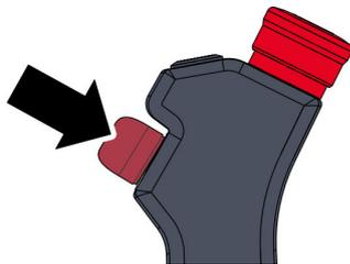
Fig. 85 Pressing the enabling button
