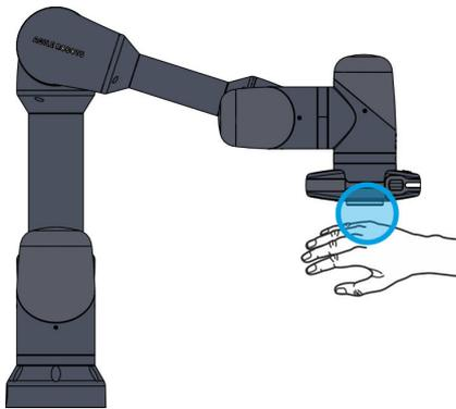
Fig. 35 Force and power limitation (example illustration)
