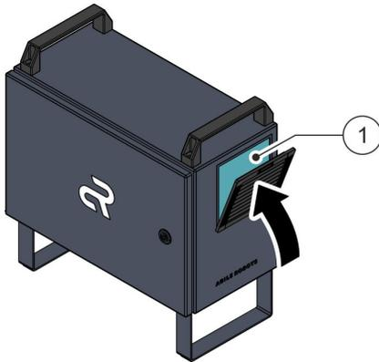
04. Close the cover on the fan filter **Fig. 90**/①.
