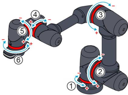
Fig. 105 Robot axes
