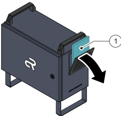
**Fig. 89** Replacing the filter unit
