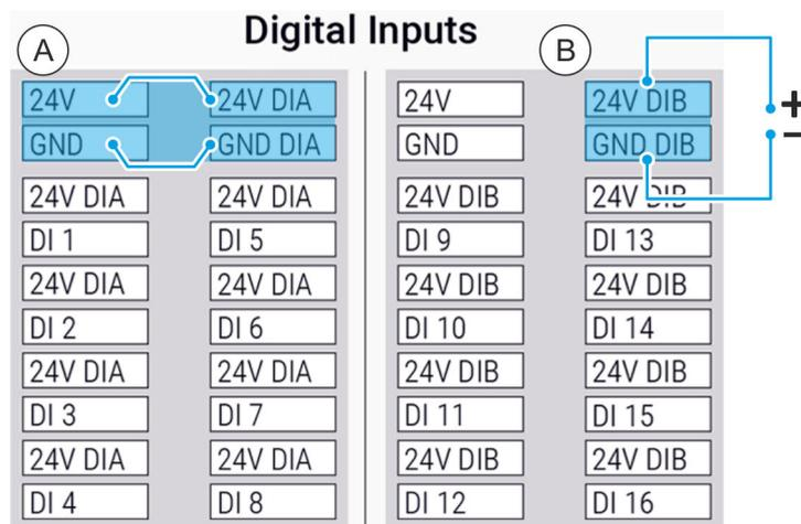
Fig. 73 Connecting the external power supply (example)
