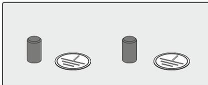
Fig. 21 Protective conductor connection points
