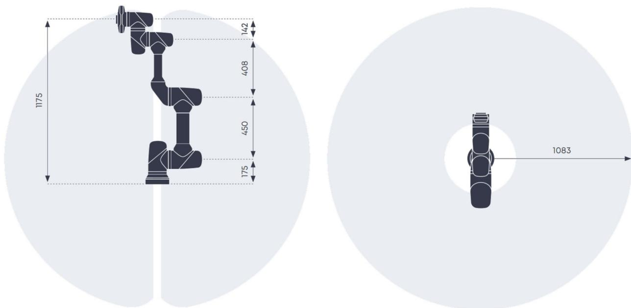
Fig. 30 Robot's working area and hazard area
