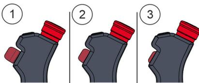
Fig. 33 Three stages of the enabling button
