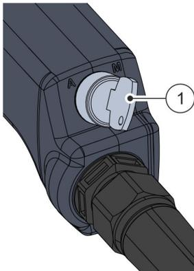
Fig. 25 Mode selector switch on the handheld controller (manual mode)
