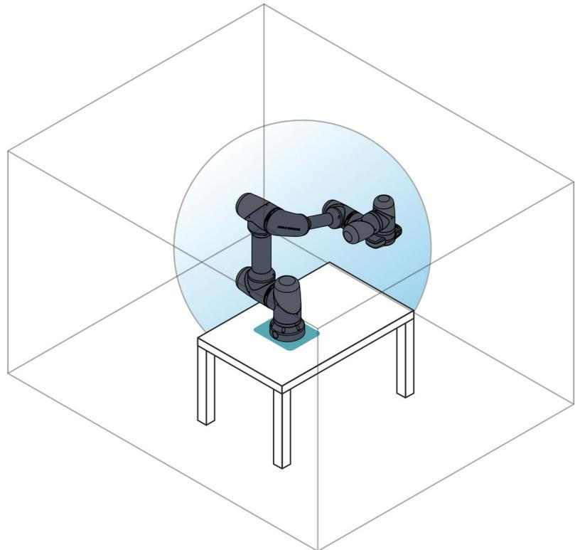
**Fig. 36** Safely limited range of motion
