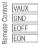
Fig. 20 Remote control interface
