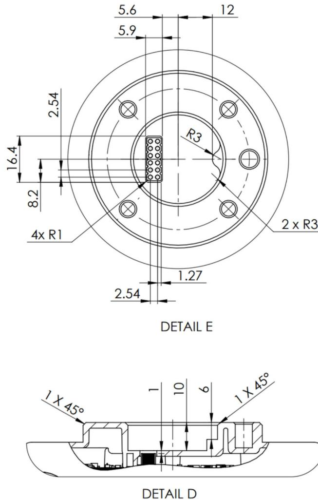
Fig. 11 Dimensions of mechanical interface on the media flange, view 2 (dimensions in mm)
