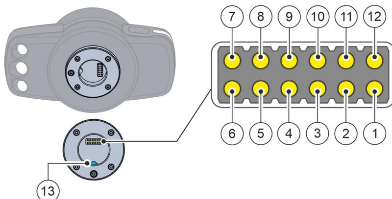
**Fig. 13** Layout of 12-pin interface
