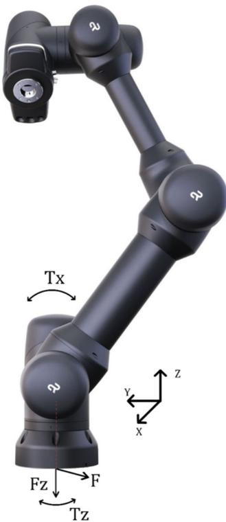
Fig. 42 Forces and torques of robot base
