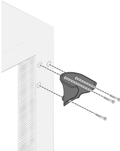
**Fig. 51** Assembling the handheld controller bracket
